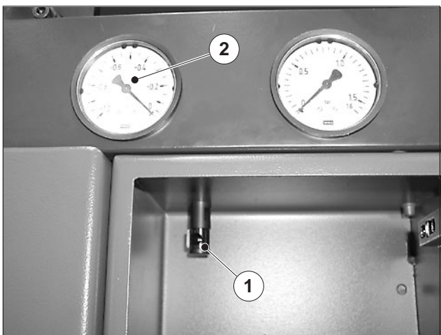
Fig. 25 Reducing the forwarding sucker suction air
