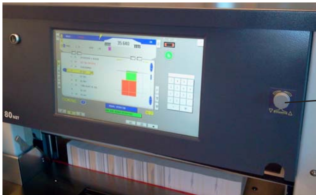
turning knob for backgauge movement (electronic hand wheel)
